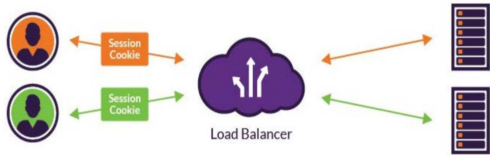
Figure 18: Sticky Routing Server Load Balancing Avi Networks Retrieved from Avi Networks from https://www.imperva.com/learn/availability/sticky-session-persistence-and-cookies/ , copyright © 2011
