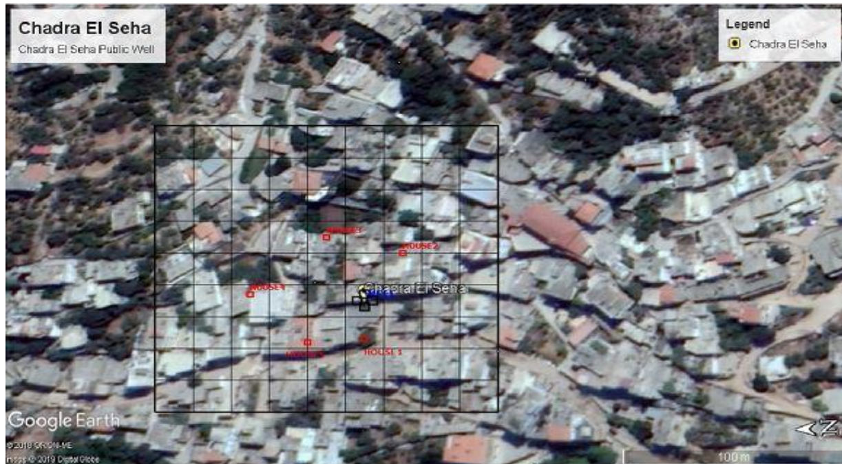
Figure 5.3: Chadra El Seha well grid - MODFLOW
