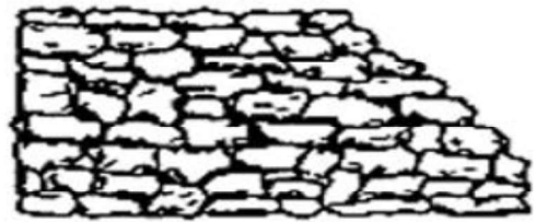
Figure 2.14 Sketch showing coursed stone wall.
