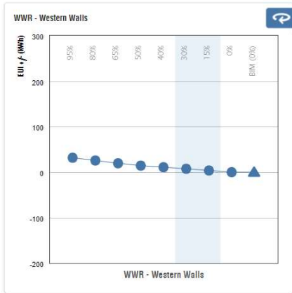
Figure B.8 Inputs of window to wall ratio for the Western walls. Source: https://insight360.autodesk.com/oneenergy/Model/201426 on: 31-05-2020
