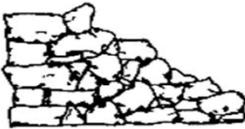
Figure 2.13 Sketch showing a random stone wall. Source: author
