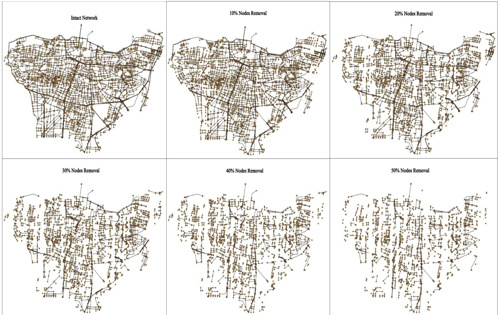
Figure 6.2: Nodal random removal of Beirut original graph with 10% interval
