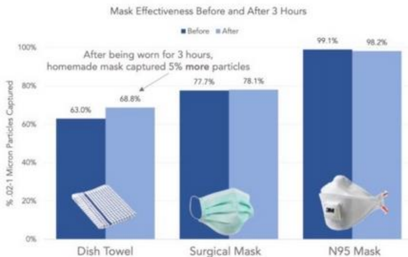
Figure 6: Efficacy comparison between homemade, surgical, and N95 mask before and after 3 hour use.(van der Sande, Teunis et al. 2008)
