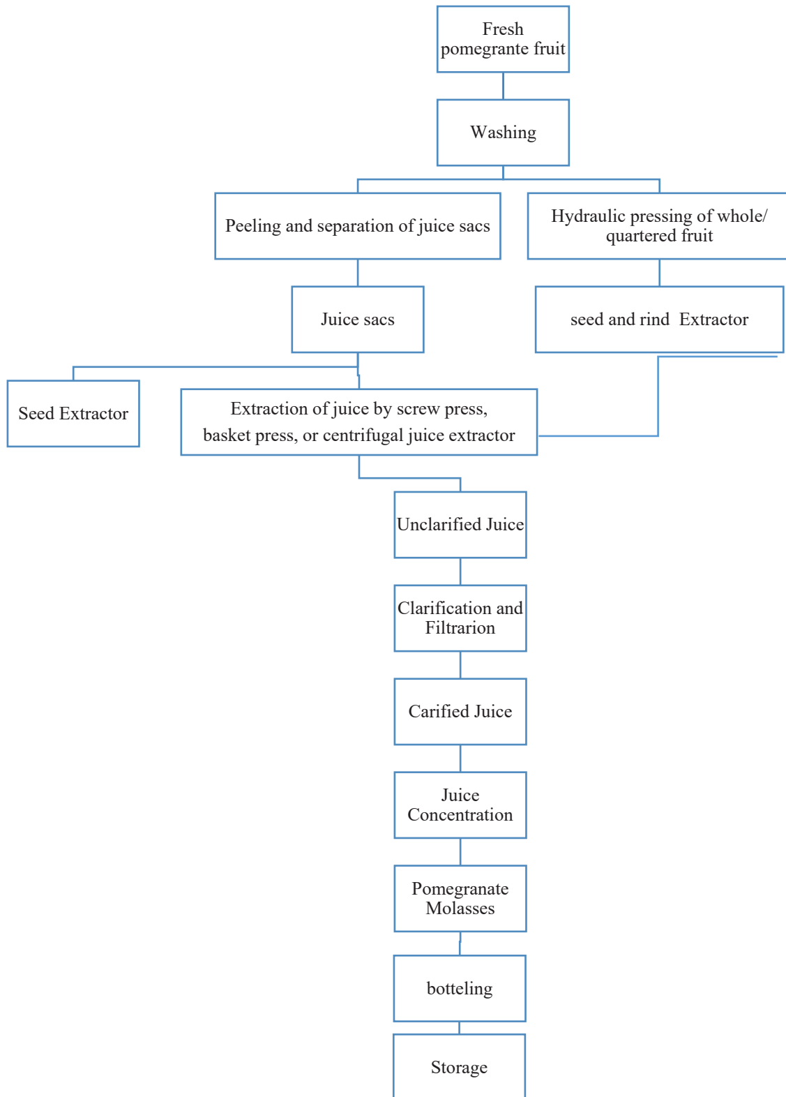
Figure 1: Production Flow Chart of Commercial Pomegranate Molasses
