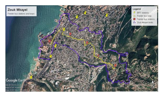
Figure 23: Proposed feeder bus stations and loops in Zouk Mkayel
