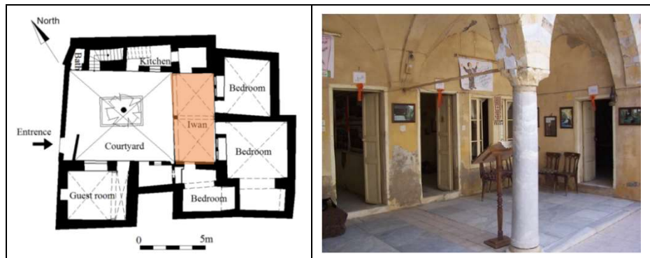
Figure 2.8(a) Plan of Ghalayini House in Gaza. (b) Perspective of the Liwan. Source: (Muhaisen, 2016) Accessed: 25-1-2021
