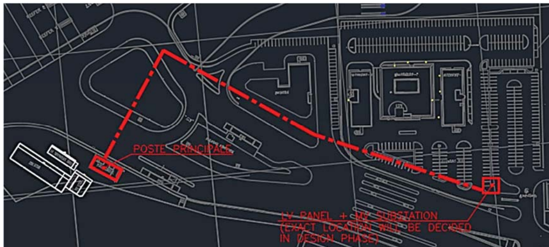
Figure 5.15 –Excavation and routing to Poste Principale
