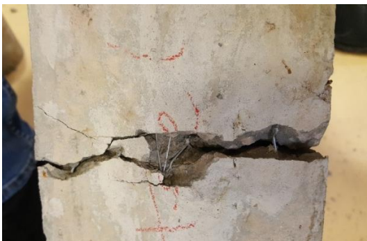
Figure 6. 31 - Failure of Concrete Specimens Retrofitted with FRC
