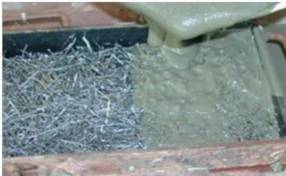
Figure 6. 8 - Slurry Infiltrated Fiber Concrete Mix
