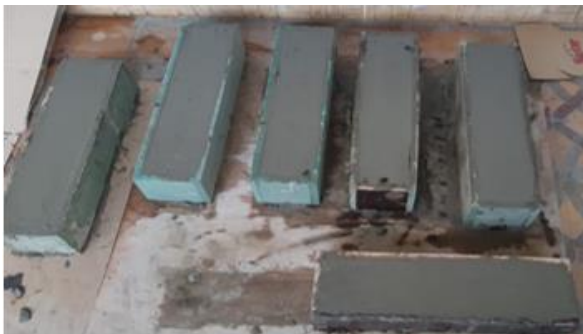
Figure 6. 10 - Concrete Beams Freshly poured
