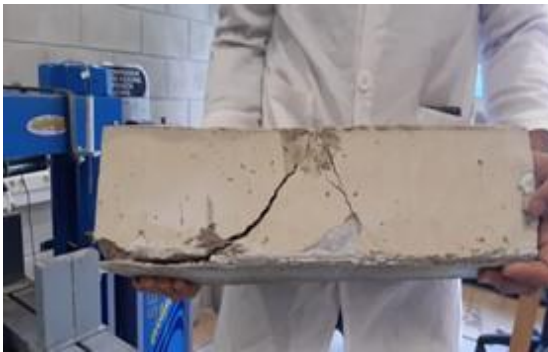
Figure 6. 30 - Failure of Concrete Specimens Retrofitted with GFRP SEH 51
