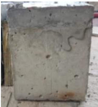
Figure 6. 20 - Concrete Specimen with FRC Hardened
