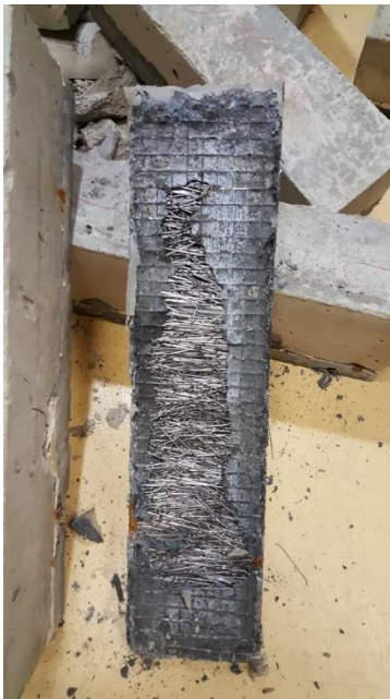
Figure 6. 32 - Failure of Concrete Specimens Retrofitted with SIFCON perpendicular
