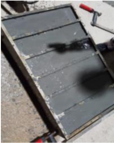
Figure 6. 19 - FRC Mix added to the Specimens
