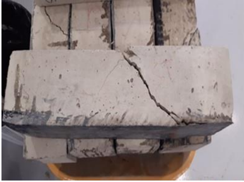
Figure 6. 29 - Failure of Concrete Specimens Retrofitted with CFRP SCH 41
