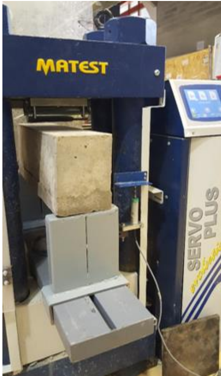
Figure 6. 2 - Specimen Supported on Roller Bearings
