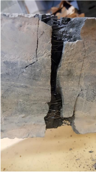
Figure 6. 33 - Failure of Concrete Specimens Retrofitted with SIFCON parallel
