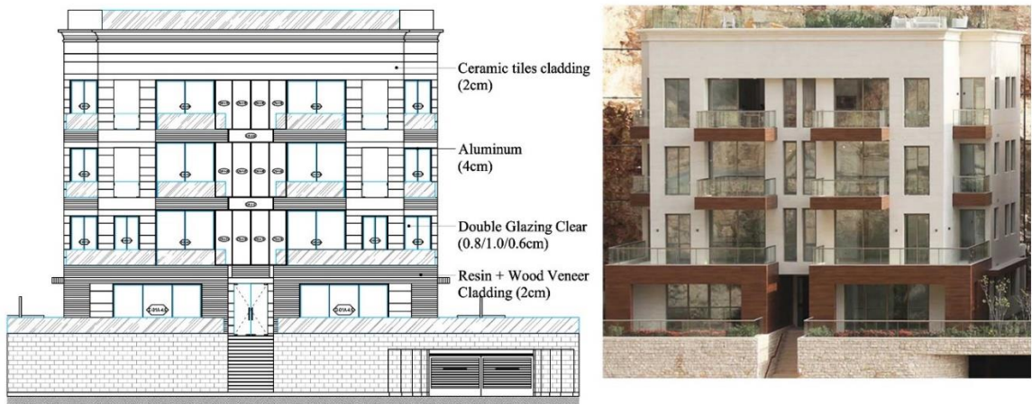
Figure 5.5: Main Elevation Drawing with materials and image of Admir - Ghazir
