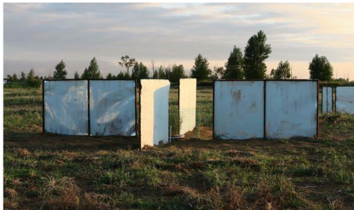
Figure 115 - Wind Baffles to help increase wind velocity around the plant (Extracted from: Zhang, 2021)
