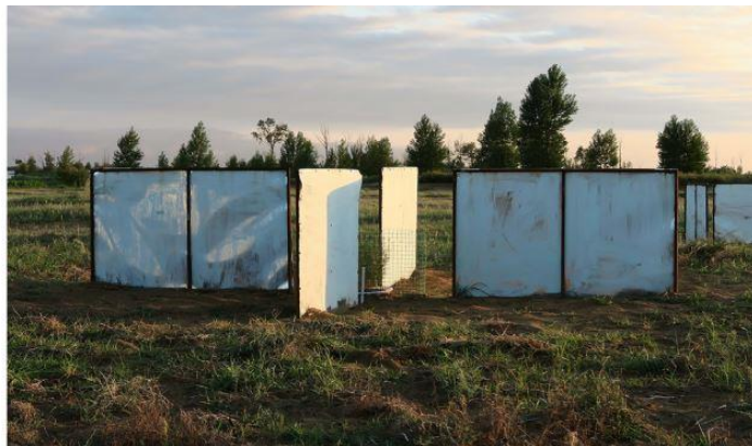
Figure 103 - Wind Baffles to help increase wind velocity around the plant (Extracted from: Zhang, 2021)
